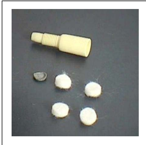
Fig. 75 old and new felt filter
