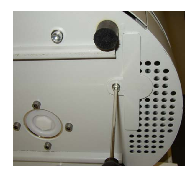
Fig. 69 Fastener for the air filter on the bottom of the leak detector
