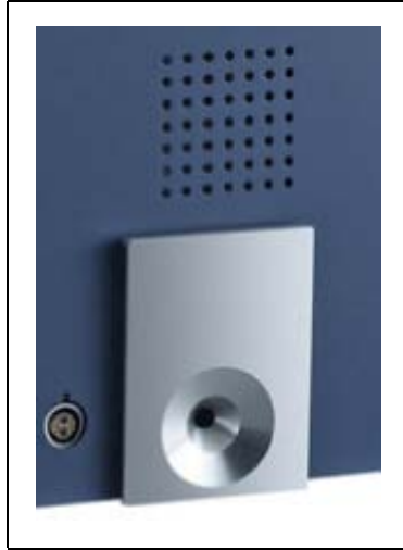
Fig. 14 Built-in PRO-Check reference leak
