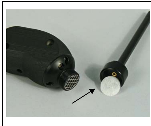
Fig. 79 Removed filter pad
