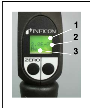
Fig. 21 Sniffer display in standard operation mode
