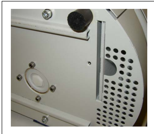
Fig. 70 Dismounting of the air filter
