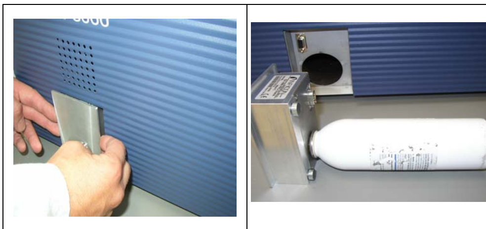
Fig. 85 Removing the PRO-Check reference leak from the main unit
