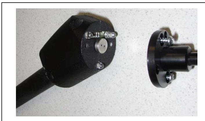
Fig. 76 Taking off the sniffer tip
